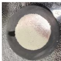
Figure A- 4: Polished sample surface of NiTi + 10% WC.
