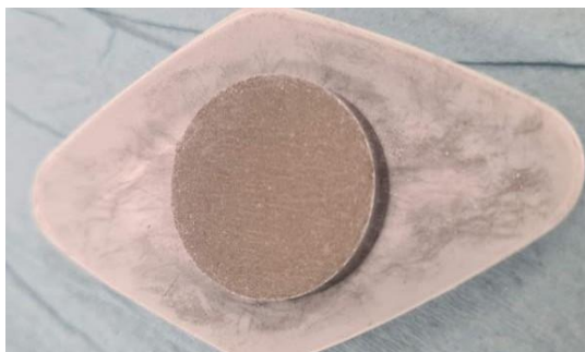
Figure A- 2: Self-mixed NiTi powder was compacted using the parameters of load 25 tons, hold time of 15 mins, mass of powder 6.5g and PVA added at 2% of the mass of the NiTi powder.
