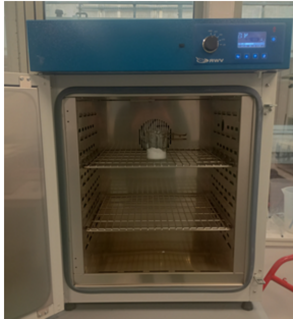
Figure 22, Inside view of Venti-line oven dryer
