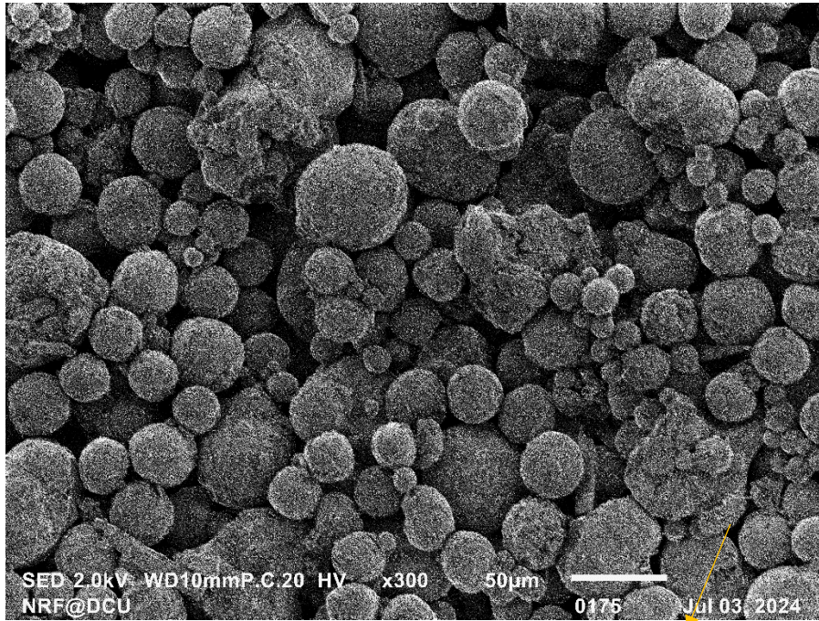
Figure 74, SEM image of HA spray coated on midrange roughness sample heat treated at 1100 °C in an air atmosphere at a magnification of 300X
