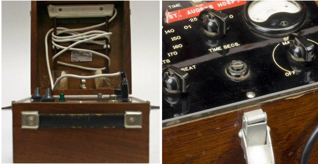
Figures 5.11 and 5.12: Left, Ectron ECT machine used in St. Davnet's, Monaghan, c. mid 1940s. 217 Right, a close-up of universal controls: an ammeter, a voltmeter and a timer. 218
