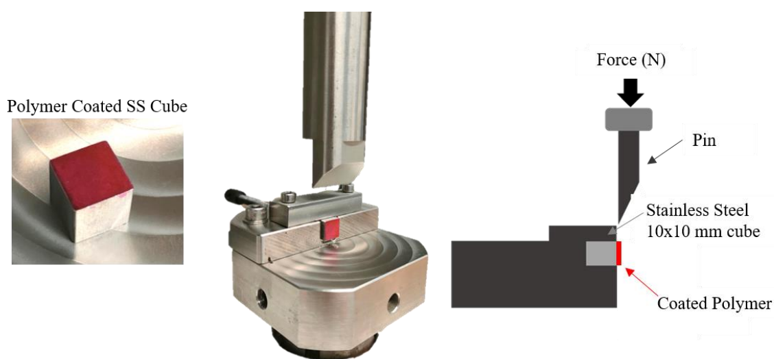
Figure 5.1: Shear Adhesion Test Set-up – Sample type and experimental arrangement used to examine the coating solutions adhesion forces on stainless steel surfaces.
