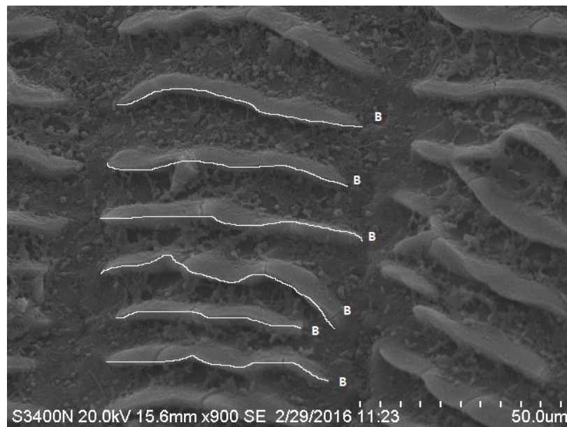
Figure 5.6. An example of a length measured by the mean of a straight line drawn from the start to the end of micro-ridge (F1) (20 kV, 15.4 mm, x400).
