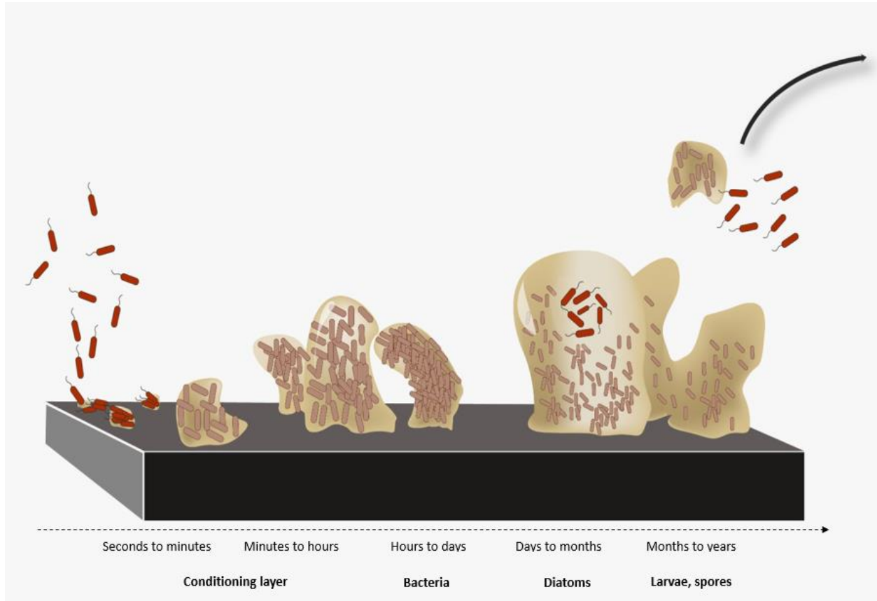
Figure 1.1. Primary steps in biofilm formation and dispersal (from left to right); a) conditioning, b) attachment, c) colonization and d) growth and detachment. The order of hard surface colonization during biofilm formation is as follows: seconds to hours (i.e., conditioning layer); hours to days (i.e., bacteria); days to months (i.e., diatoms) and months to years (i.e., larvae, spores) (Adapted from 1 ).
