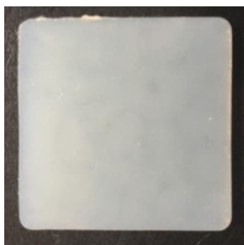
Figure 4.58 Cured PP-B-T20-M-M9-8; no amount of voids present
