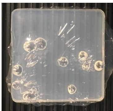
Figure 4.45 Cured PP-B-T20-M-M8-1 with voids in sample
