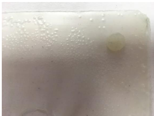
Figure 4.39 Visible bubbles in cured in cured PP-B-T20-M-M6 after an 8-hour cure at 100°C
