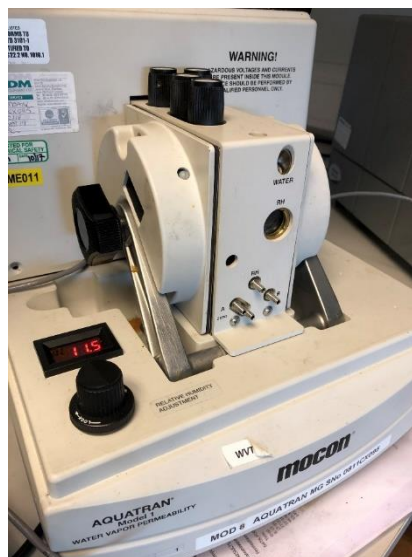
Figure 3.18 AQUATRON Model 1 from MOCON for water vapour transmission rate testing
