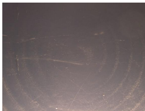
Figure 4.34 PP-B-T20-M-M5 with 25% heptane and increased number of evacuations, first void free sample, Figure 4.33 magnified
