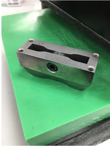
Figure 3.8 Qualitest Die used to cut tensile samples
