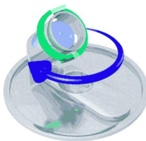
Figure 4.16 Representation of the dual asymmetric mixing employed by the Speedmixer DAC 50.1 FV
