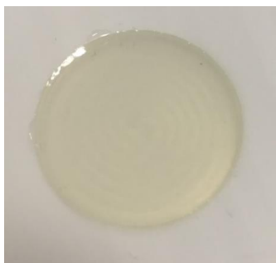
Figure 4.33 PP-B-T20-M-M5 with 25% heptane with increased number of evacuations, first void free sample
