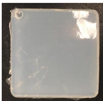
Figure 4.53 Cured PP-B-T20-M-M9-5; small amount of voids present
