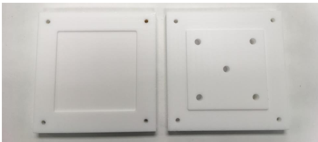
Figure 4.35 Water Vapour Transmission Mould made of PTFE. Uncured PIB-PUR is placed on the female section on the left. Male section on right is secured in place with allen key screws
