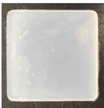
Figure 4.52 Cured PP-B-T20-M-M9-4; no voids present
