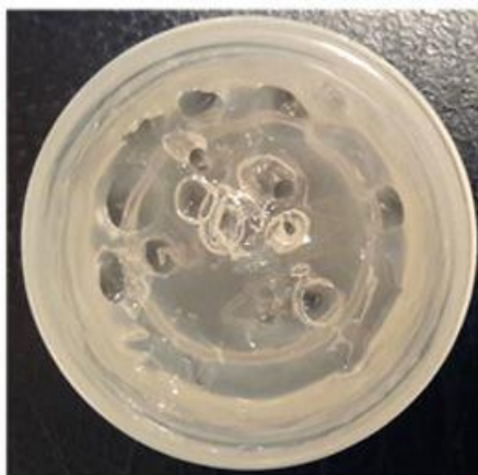
Figure 4.21 PP-A-M-M3 evacuated at 50°C to 0 ATM 21 times
