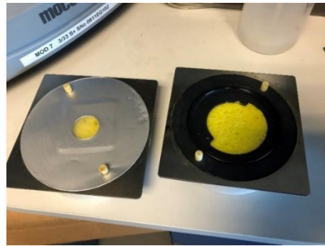
Figure 3.17 PIB-PUR material in sealed aluminium mask sitting in open diffusion cell
