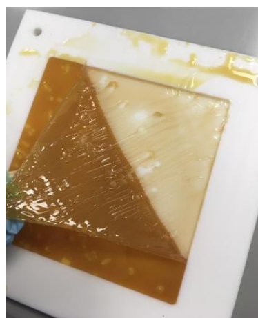
Figure 4.42 PP-B-T20-M-M7 evacuated at 100°C for 3 hrs, cured at 100°C for 15hrs and cured at 150°C for 15hrs was uncured after 24 hours in oven displaying a dark colour suggesting burning and tacky underside, suggesting insufficient curing
