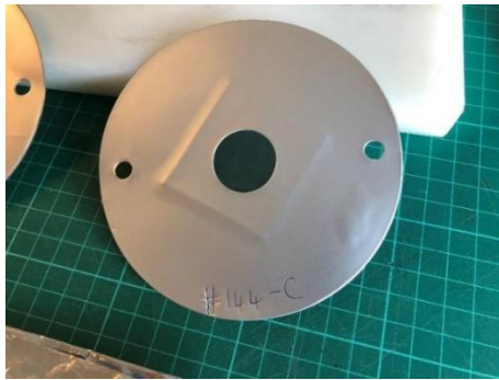
Figure 3.16 Aluminium mask enclosing PIB-PUR material prior to test WVTR
