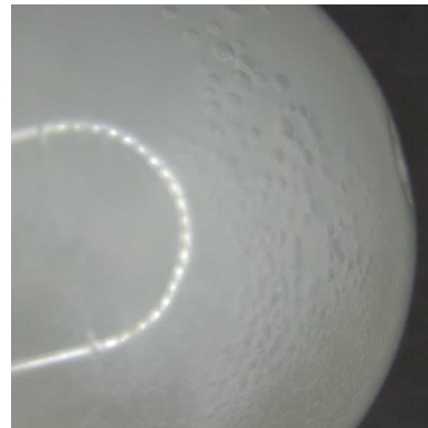
Figure 4.26 Uncured PP-A-M-M4 after centrifuging at 4000 rpm for 1.5 hours
