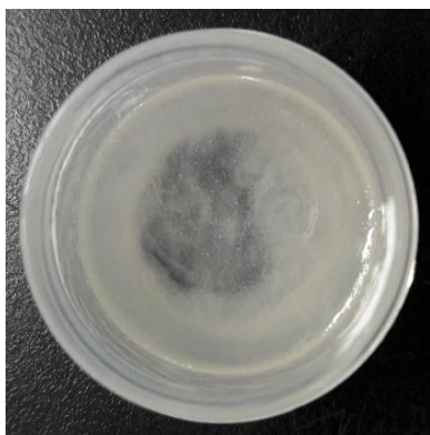
Figure 4.23 Uncured PP-A-M-M4 mixed at 3500 rpm for 10 mins in 25 mm diameter tub prior to centrifuging
