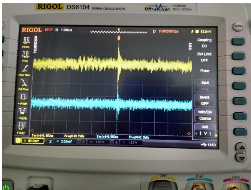
Figure 38 Screenshot of Real time E- and B-field Acquisition on the Oxford Instruments PlasmaLab 100 CCP - Forced Arcing. The B-field signal is shown in blue; the E-field signal is shown in yellow.
