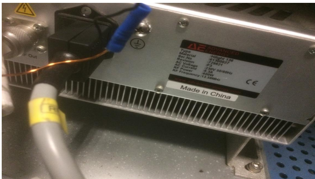
Figure 92 Oxford Instruments PlasmaLab 100 Tool RF Power Supply Unit
