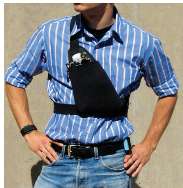
Figure 2.4: The "InSense" system developed at MIT stores data on a PDA contained within the pack Source: Blum, Pentland, & Troster [22].
