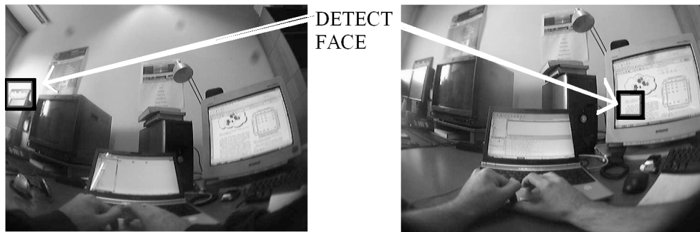
Figure 5.7: An example of an error by the face detection technique on user 3 from table 5.1.
