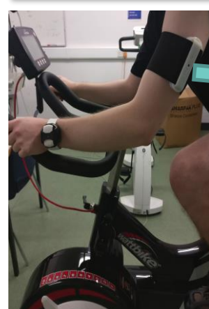
Figure 6: The watch and pod like 'SwEatch' platform placed on the volunteers wrist and upper arm during trials
