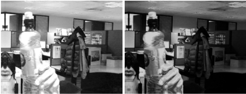
Figure 2-5: Example of the vignetting effect. The image on the left side does not have vignetting effect. The image on the right side shows a light vignetting effect. It can be seen that the pixels in the middle are brighter than the rest for the right image. For visualization purposes the image with the vignetting effect has been manually edited to enhance the effect.
