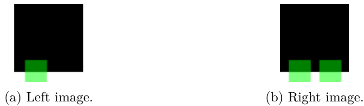
Figure 2-3: Illustration of the aperture problem. The green rectangle is the search neighbourhood on the left image. It is not possible to identify which of the two rectangles on the right image corresponds to the one in the left image by using only pixels contained in the neighbourhood defined by each rectangle.
