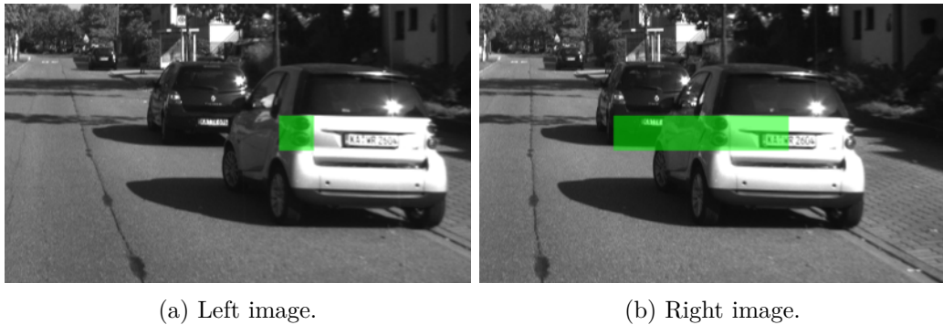
Figure 2-6: Example of the search range for a local approach. The green square on the left image represents the search pattern, the green rectangle on the right image represents the search area.
