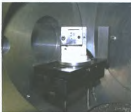
Figure 3.23: Mount 1, for EUV studies, this mount would be used to position baffles, to 'catch' debris from the laser-plasma, and also to lesson the pressure wave which is generated during ablation, which travels down the length of the spectrometer. This can cause arcing of the EUV detector when the laser is firing at a high repetition rate.
