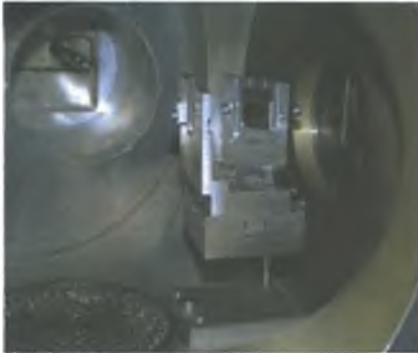
Figure 3.24: Mount 2. Used to position the probe array arm, independent of the main target table, but also capable of mounting internal optics.
