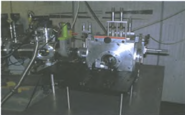
Figure 3.19: EUV/VIS/probe vacuum chamber mated to EUV spectrometer (left hand side of photograph). The chamber is made from aluminum, a cube of side 24.5cm and internal volume of approximately 5440\text{cm}^3 . It is equipped with six flanges, each configured for different experiments.
