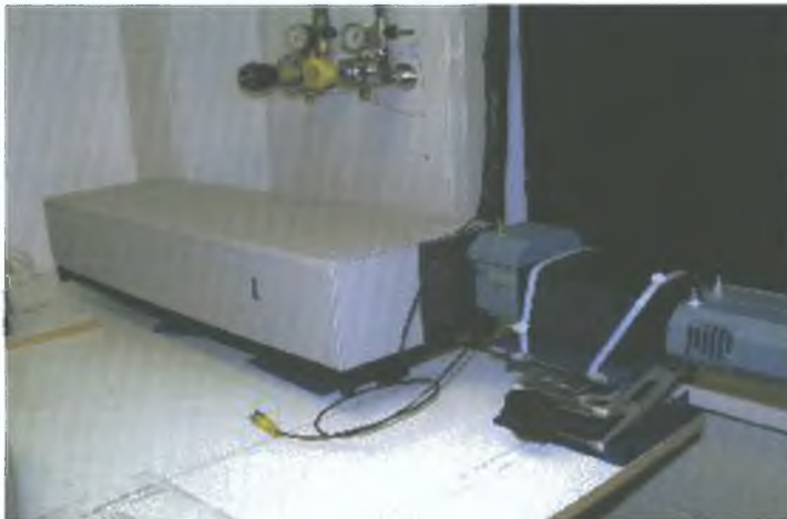
Figure 3.8: Chromex 0.5m Visible spectrometer, mated to the Andor ICCD camera. Direct connection to the ICCD head allowed the head to be gated directly from a Stanford delay generator.
