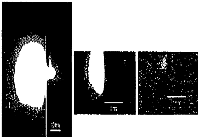
Figure IV XUV images (pin hole camera gate time, 2nsec) from Z. Andreic et al [1]. The first image (far left) is taken at 10nsec, the second (middle) is after 18nsec, the third 58nsec (right) after the laser pulse. In all cases the laser came from the left.
