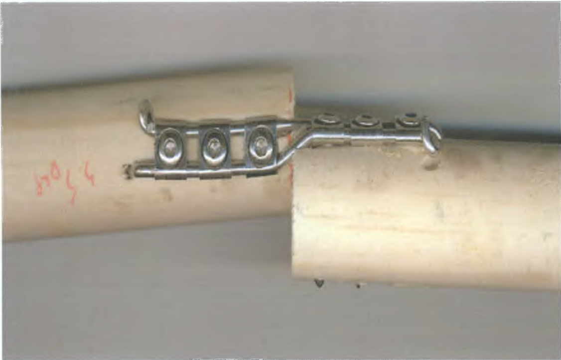
Fig. 6.26 2.4/3.5 fd Torque Failure
