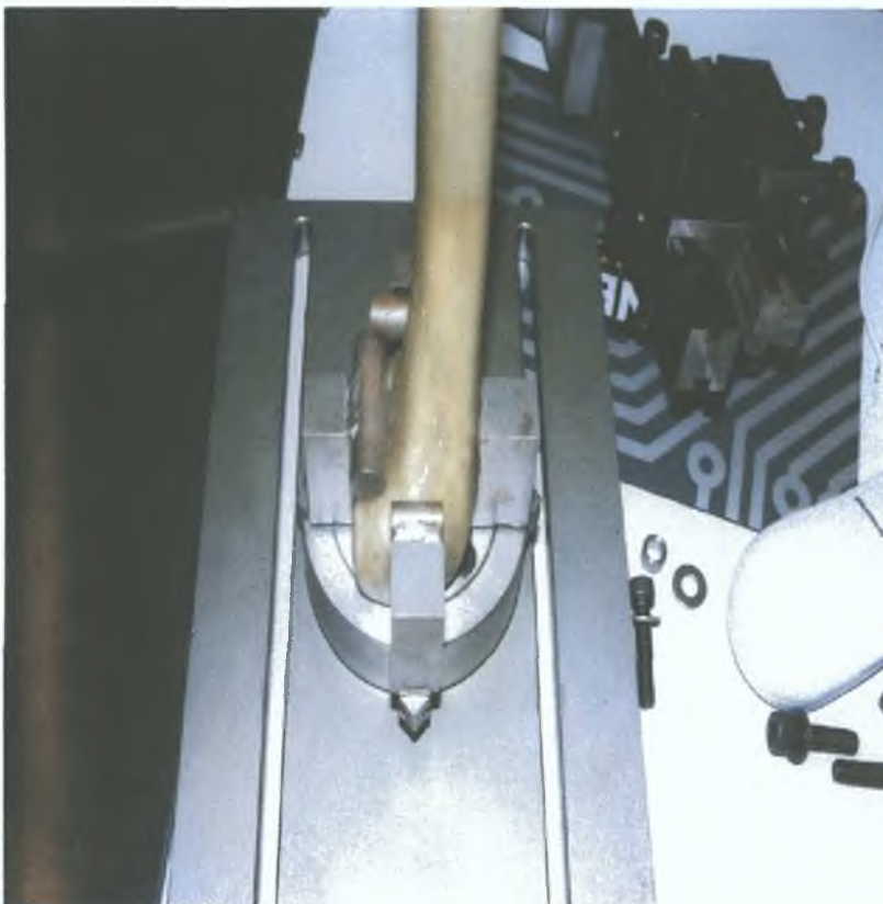
Fig. 8.3 Close up of grips used to hold distal femur
