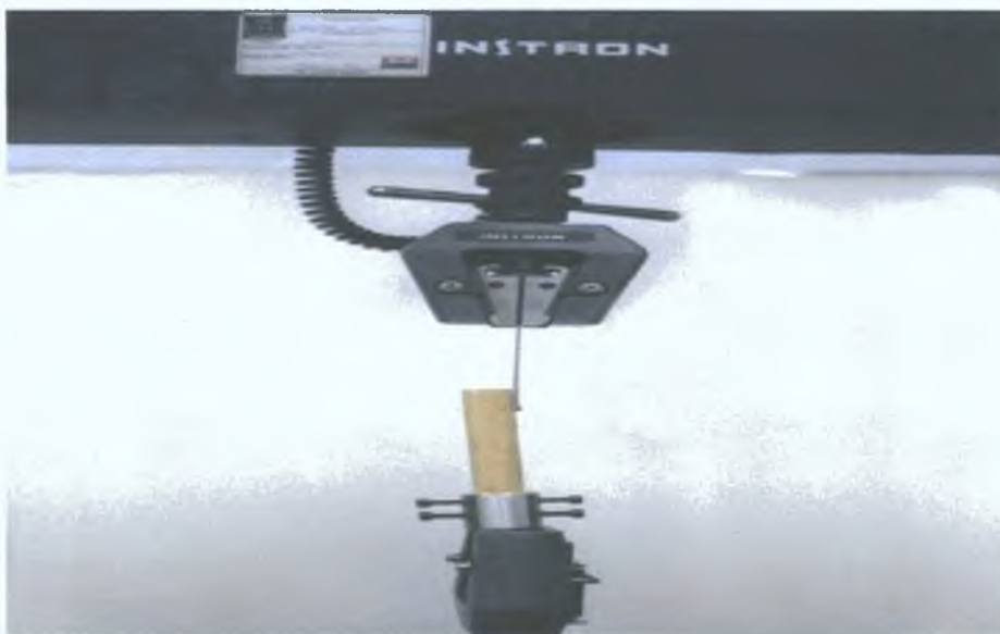
Figure 3.7 Tensile Testing of a Prepared Sample
