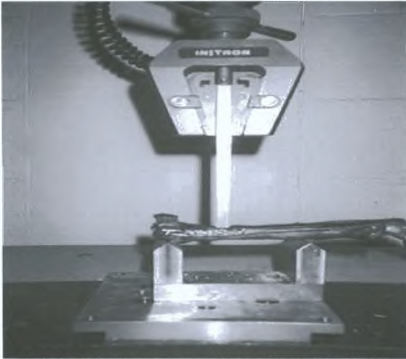
Fig. 7.1 3-point bending of canine distal radius repaired with 1.6/2.7Fd
