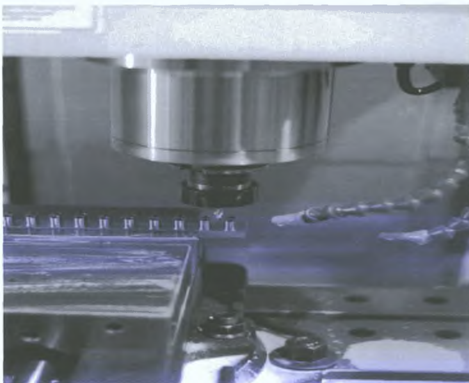
Fig. 5.3 Machining outside profile and creating holes
