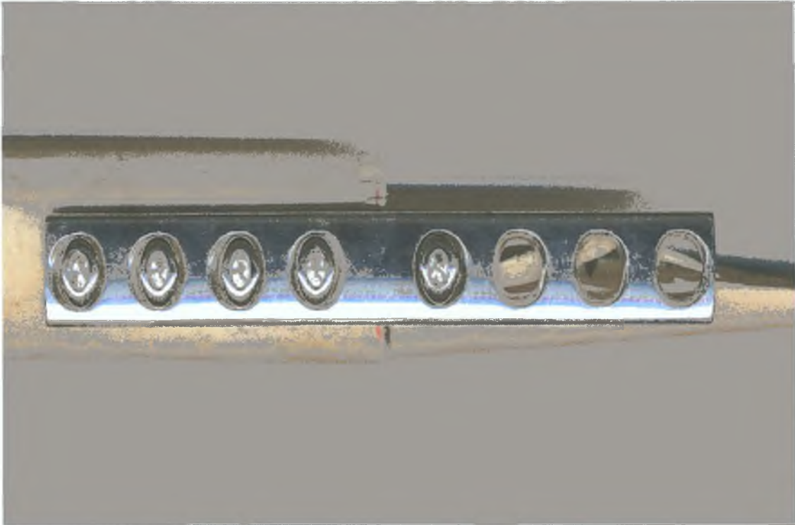
Fig. 6.28 Narrow 4.5 DCP Torque Failure
