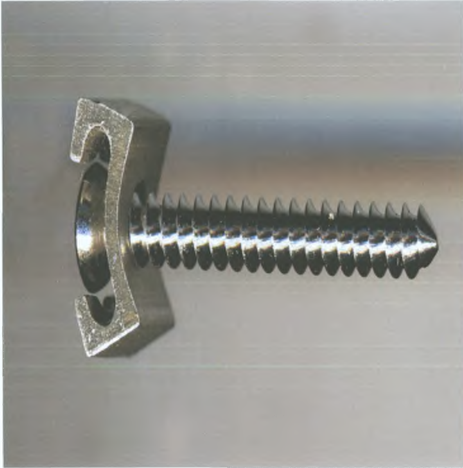
Figure 3.26 Close up of a clamp showing the opening out like a flower because of four point bending resulting in loss of contact between the screw head and pins
