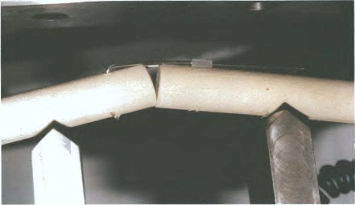
Figure 3.11 A Type 3 clamp undergoing four point bending
