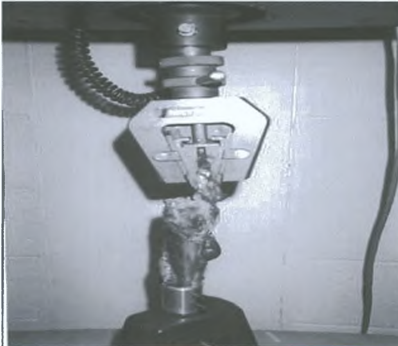
Fig. 7.2 Tensile testing of canine tibial tuberosity top clamp on patella
