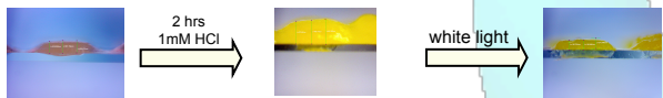
Ionogel in the initial state (left), after 2 hours in HCl (centre) after white light irradiation (right).
