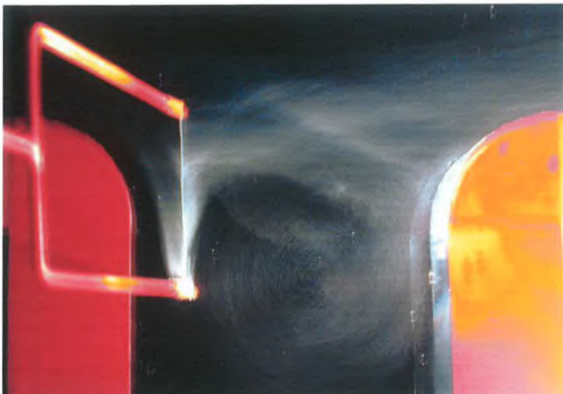
Figure 5.37: Entry flow patterns for a round entry 50*50mm equal tee at 0.5 m/s.
