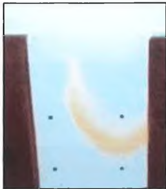
Figure 5.17: Fluid movement along the downstream wall of the branch
