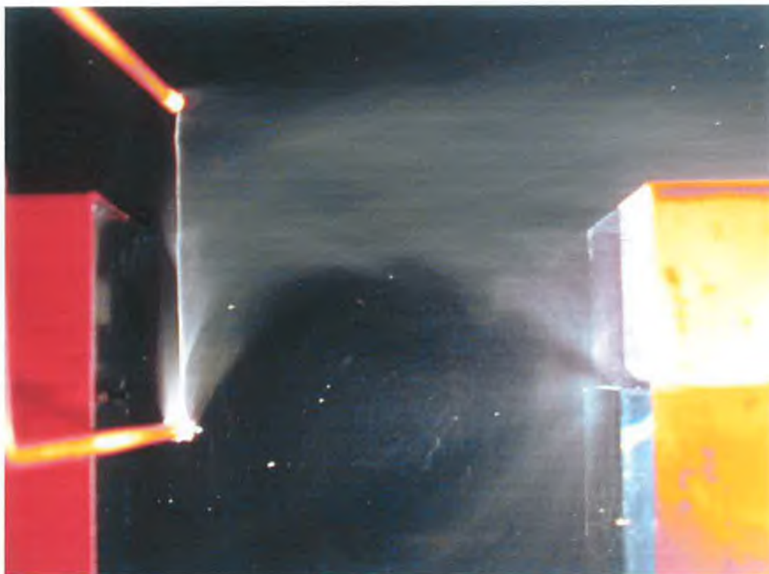
Figure 5.28: Mainstream flow for a 50*50 sharp entry tee at 0.5 m/s
