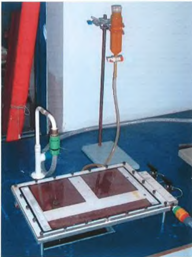
Figure 5.2: Dye injection bottle and flow plate
