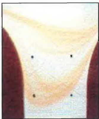
Figure 5.19: Long radius bend mainstream flow penetration
