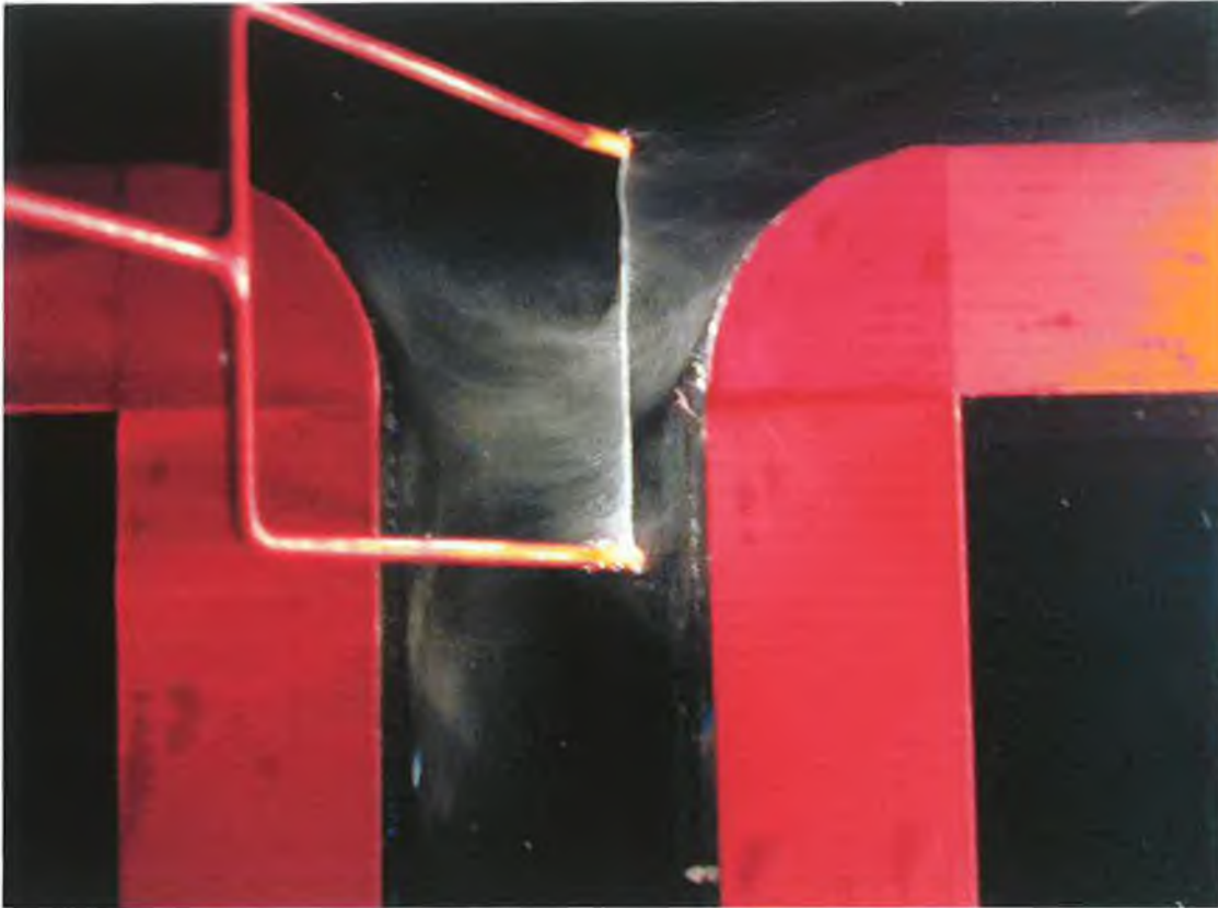
Figure 5.46: Sharp entry re-circulation in a 50*25 mm dead-leg tee at 0.5 m/s
