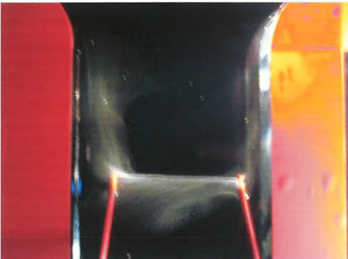
Figure 5.40: Midstream separation for a 50*50mm equal tee at 0.5 m/s.
