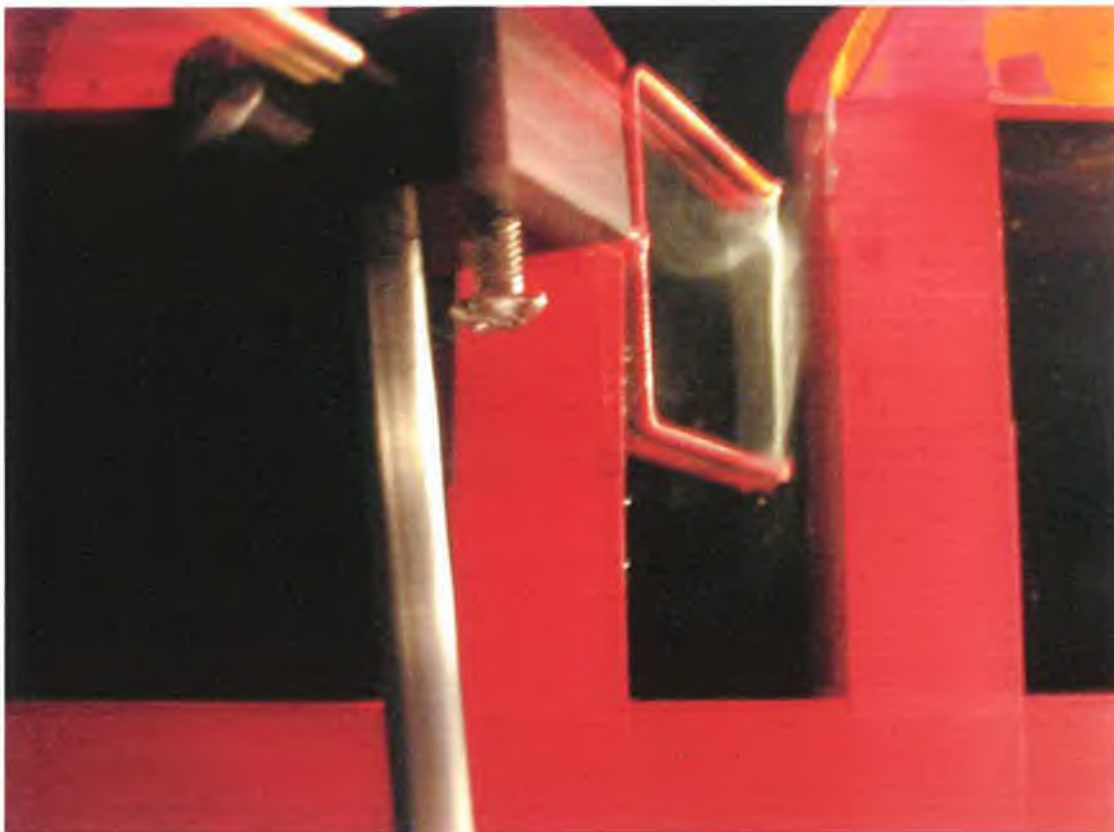
Figure 5.47: Downstream flow patterns in a 50*25 mm dead-leg tee at 0.5 m/s
