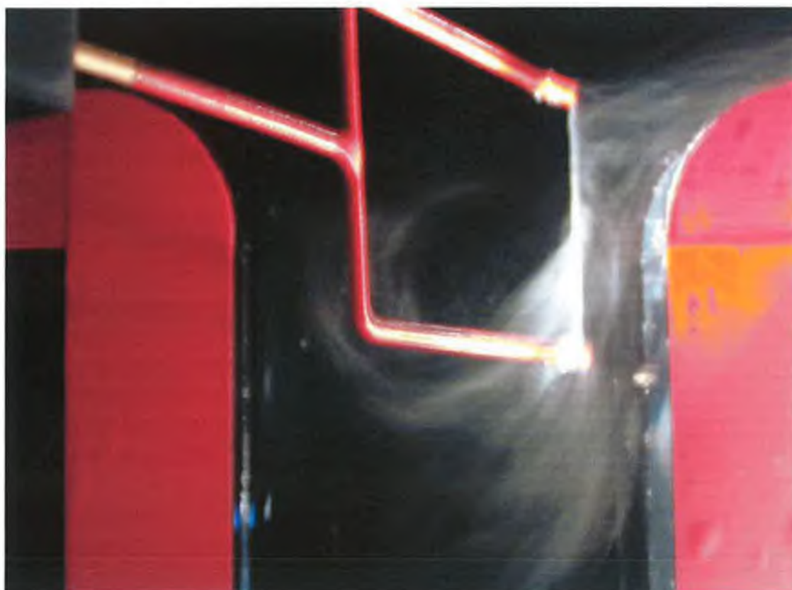
Figure 5.38: Downstream patterns for a round entry 50*50mm equal tee at 0.5 m/s.
