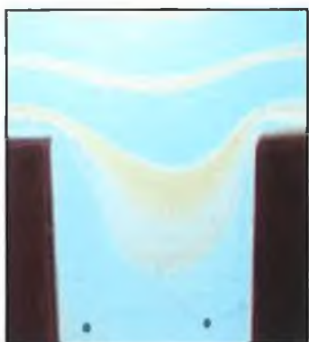
Figure 5.15: Mainstream flow branch penetration
