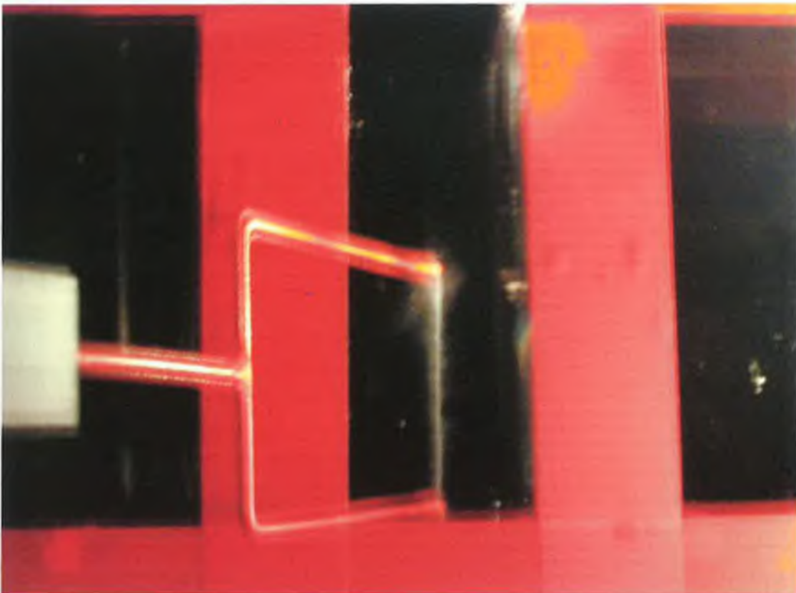
Figure 5.45: Stagnation at the base of a 50*25 mm dead-leg tee at 0.5 m/s
