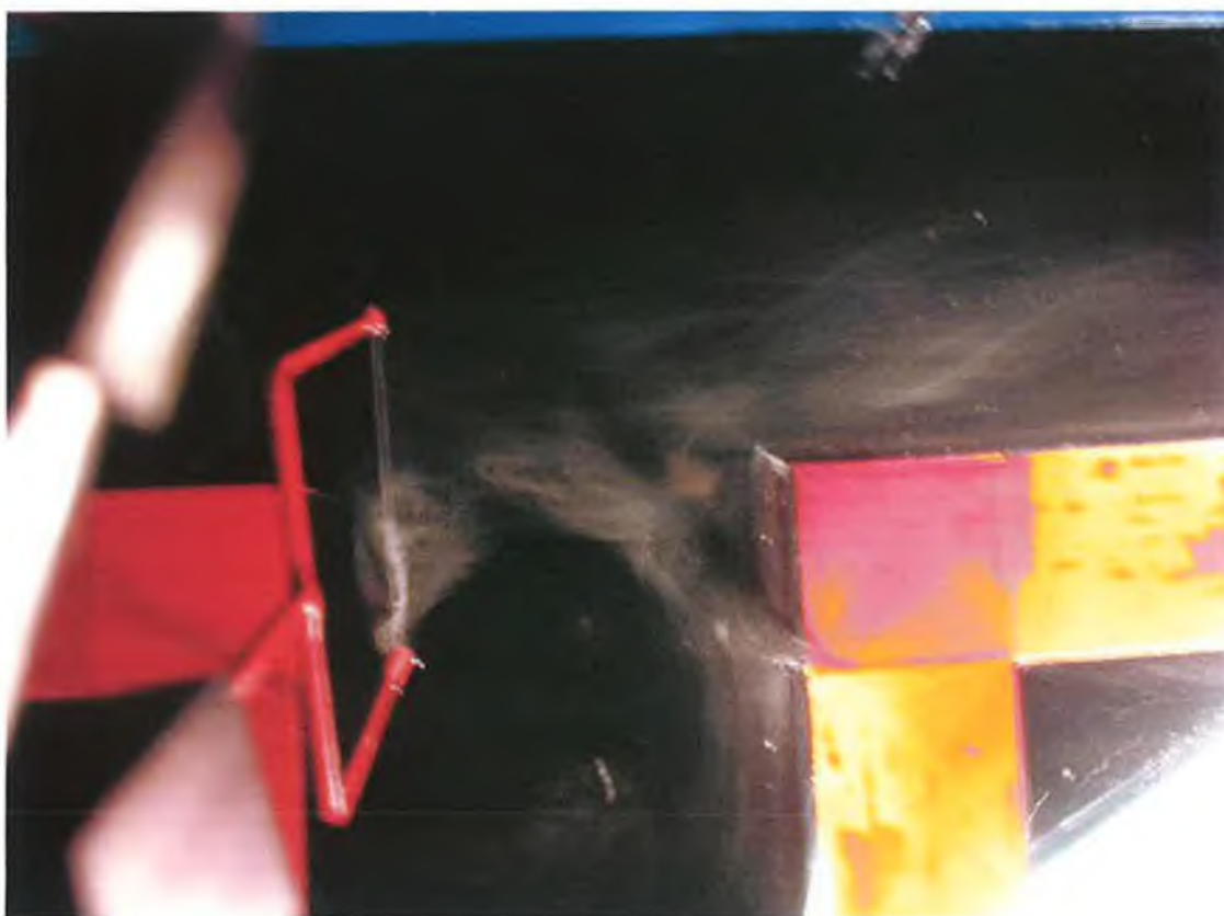
Figure 5.29: Downstream separation for a 50*50 sharp entry tee at 0.5 m/s
