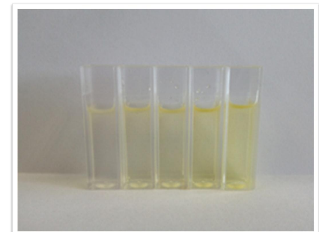
Fig 10: Cuvettes showing the change in colour intensity of nitrate samples with chromotropic acid.
