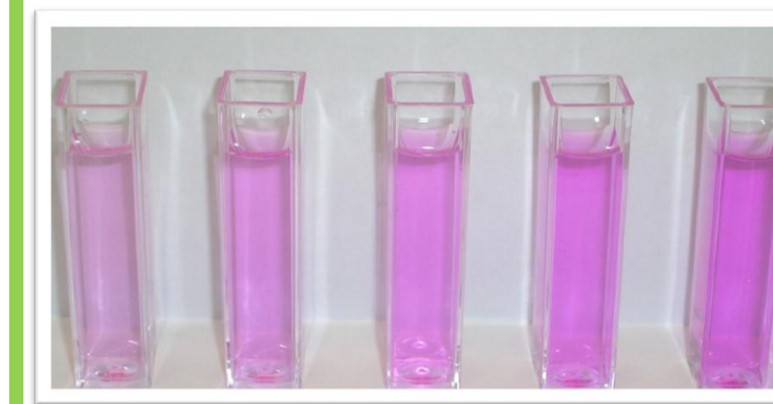
Fig 8: Cuvettes showing the change in colour intensity of nitrite samples with Griess reagent.
