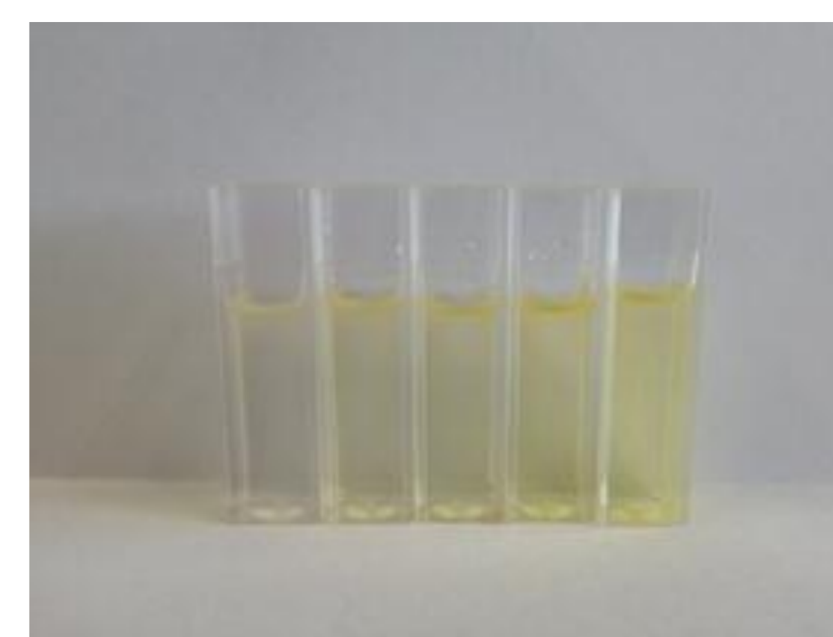
Fig 8: Cuvettes showing the change in colour intensity of 0.5 - 3.5 mg/L nitrate samples with chromotropic acid reagent.
