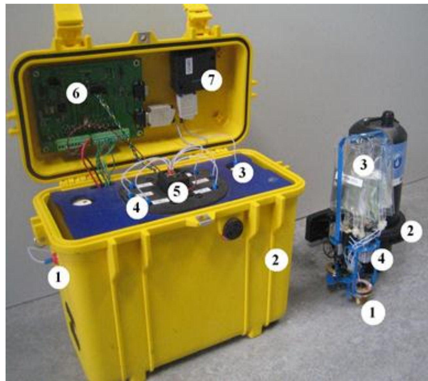
Fig 1: First and second generation phosphate systems. (1) Sample inlet; (2) IP68 Enclosure; (3) Reagent storage; (4) Pumps; (5) Microfluidic detection system; (6) Control board; (7) Communications.
