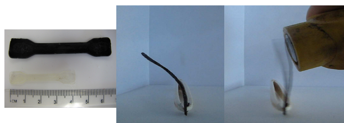
Fig. 3. Left: Dry ionogel and swollen ionogel loaded with magnetic particles; Right: Response of the magnetic ionogel to an external magnetic field
